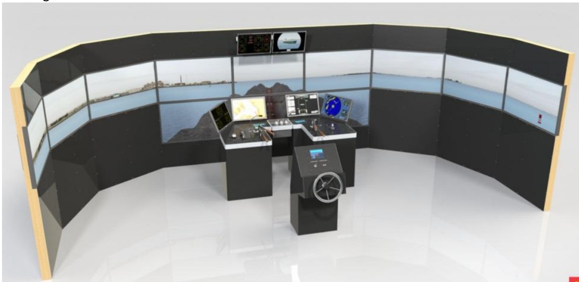
Figure 11: Class A - Full mission inland navigation simulator example
