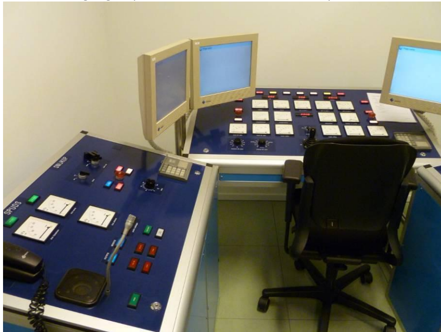
Figure 13: Class S - Special task inland navigation simulator example
