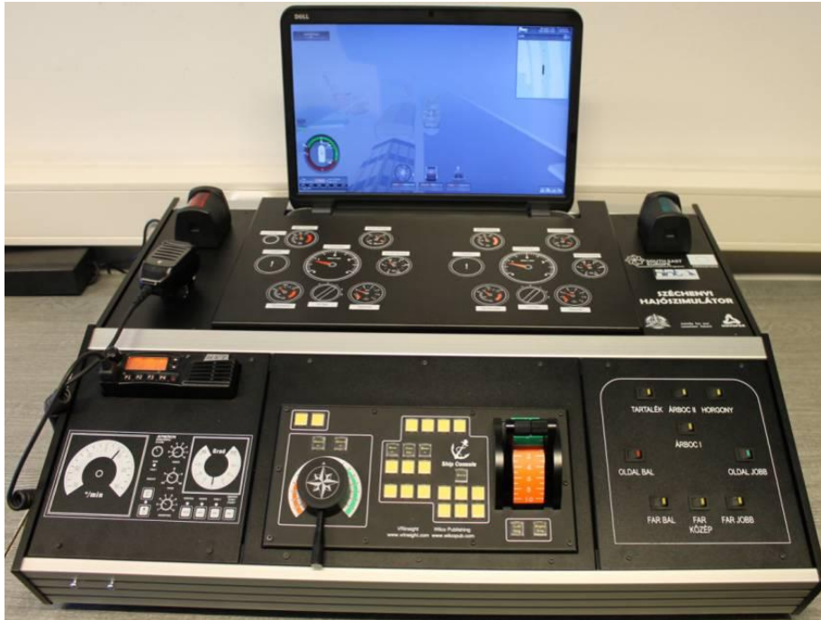
Figure 7: Class E - Exhibition inland navigation simulator example
